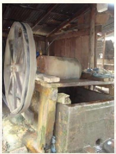
Step 1: Grind ore with rod mill/ball mill without using mercury
