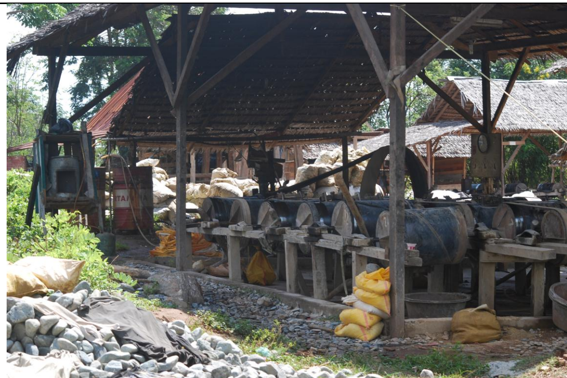
Figure 4. When the gold price was peaking up, more than 20,000 units of ball-mills were working 24 hours. Less than 20 plants obtained business permits and Environmental Impact Assessment reports from the Environmental Agency of Palu City. In June 2011, mercury vapor in this area measured as high as 45,000 ng/m 3 . Photo: Yuyun Ismawati/BaliFokus.
