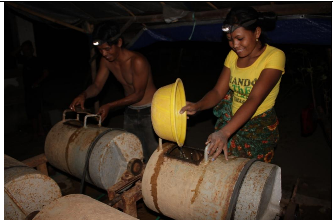
Figure 9. A young woman working in the ball-mills unit, exposed to mercury during the process day and night. Most of the ball-mill units have no permit. Photo: Baiq Dewi Krisnayanti.
