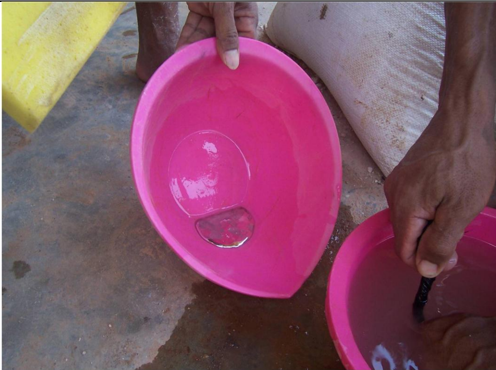
Figure 5. About 500 gram mercury are added to each ball-mill and mixed for 5 hours. At the end of the process, the amalgam is formed and brought to the gold shop to be burned. Photo: Yuyun Ismawati/BaliFokus.
