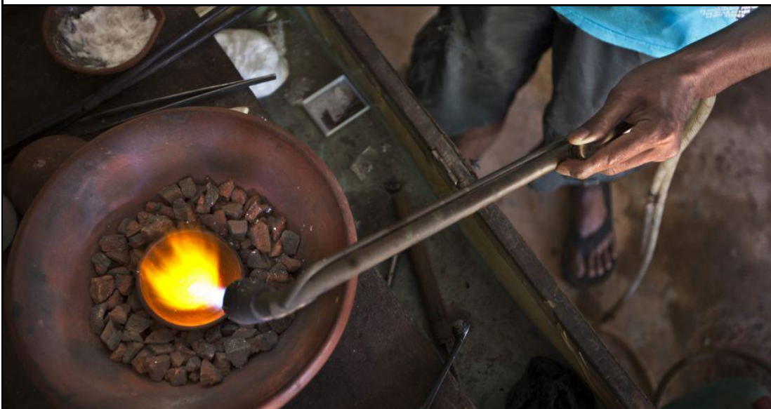
Figure 10. Workers burn the crushed ore, which has been mixed with mercury, hoping to capture flecks of gold. Mercury vapor would last in the air for 1-1.5 years. Photo: Kemal Jufri/The New York Times, 7 July 2011. http://www.nytimes.com/2011/07/08/world/asia/08indo.html?pagewanted=all&_r=0
